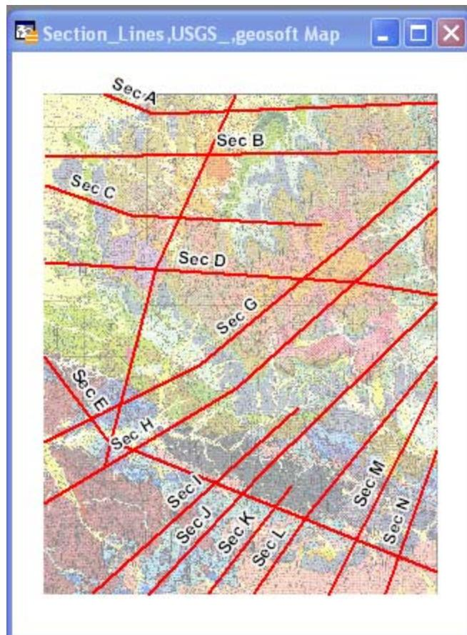
A MapInfo table containing polylines representing the position of each cross-section is also required. Each polyline must be attributed with the cross-section image file name and the **Top** and **Bottom** elevations of the image. An example is displayed below.
